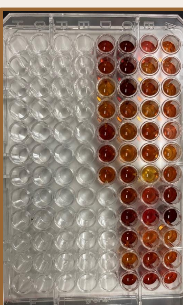
Figure 5: Microplate with tannin samples. Samples would turn this darker color once heated.
